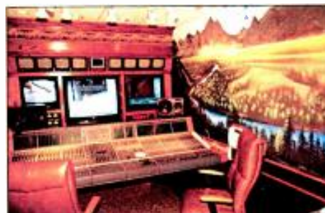
TNN is using an AMS Neve digital audio console in its new audio-only remote truck.
